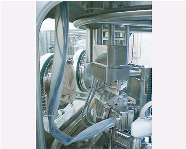
图5 GKF HiProTect 1700上X光样机 (来源: 博世)
